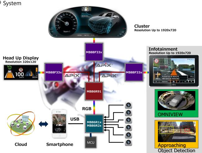
Note: APIX stands for **A**utomotive **Pix**el Link APIX is a Point-to-Point Video and Data Link optimized for Automotive environment provided by Inova Semiconductor, which is Headquartered in Munich, Germany.
