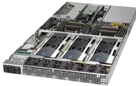
Figure 6. High Density 1U Server for the Data Center supporting up to 32 UHD or 128 FullHD HEVC ABR Bundles
