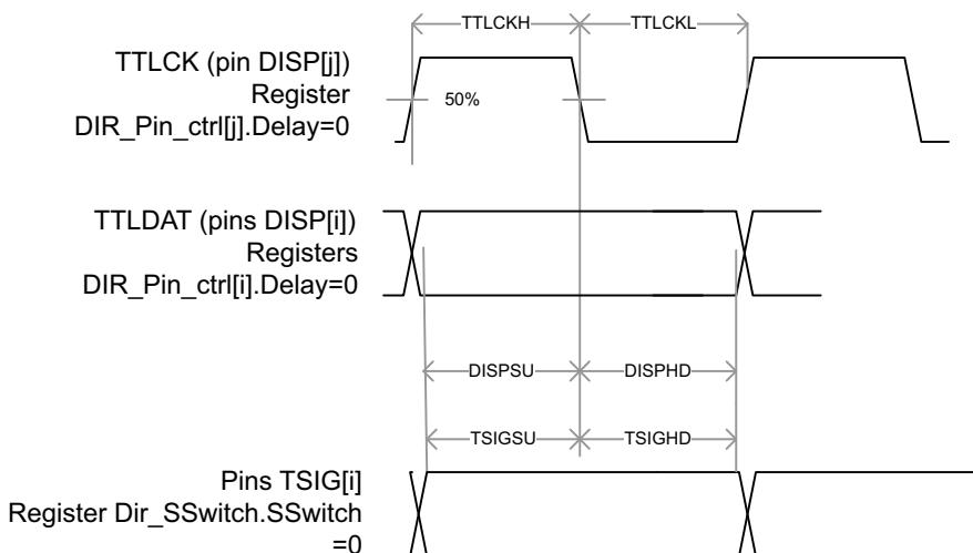
**Figure 2.27. :** TTL operation output timing (1)
