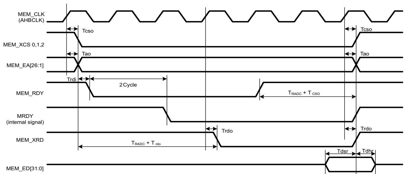
**Figure 2.13. : Low speed device Read**
