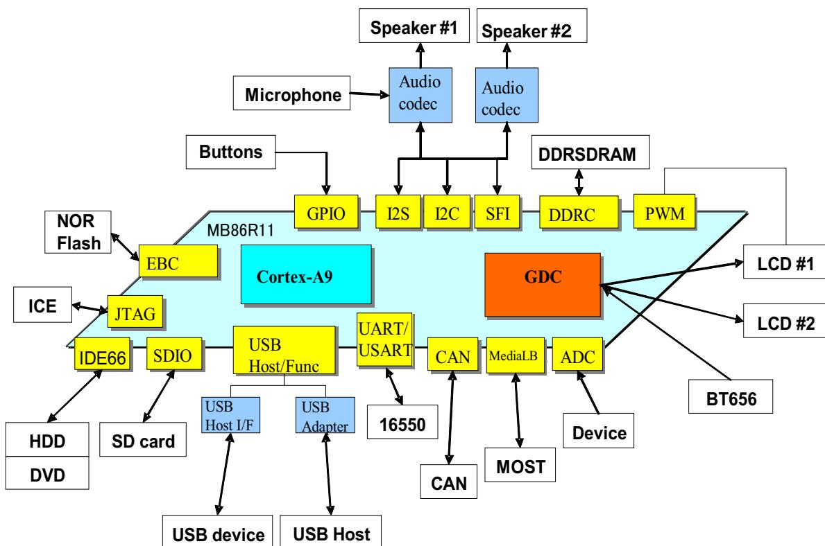
**Figure 1.4. :** MB86R11F system configuration
