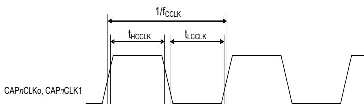
**Figure 2.30.** : Video capture clock input signal timing
