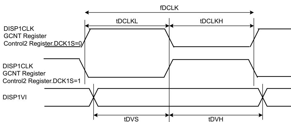
**Figure 2.29.** : ITU-R BT656 Display Timing
