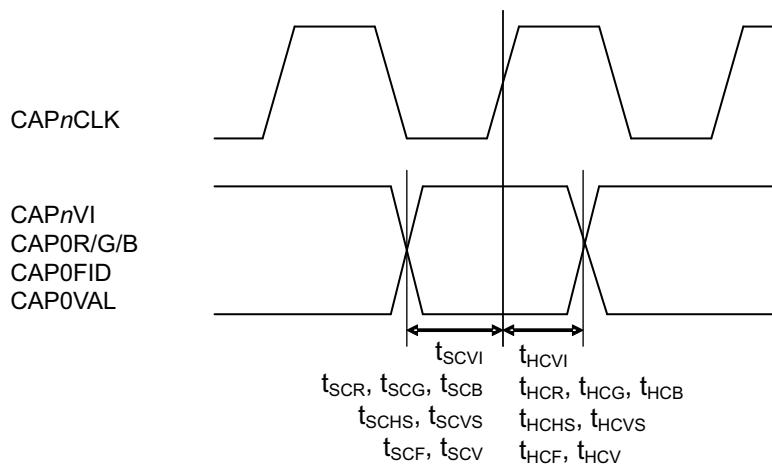
**Figure 2.31. :** Video capture input signal timing
