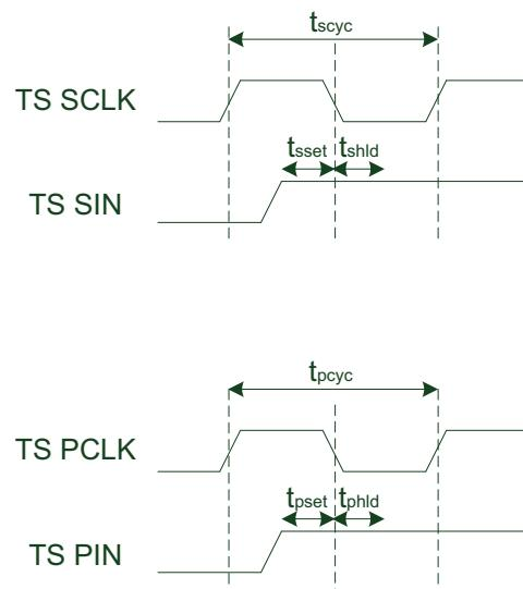
**Figure 2.51.** : TS timing of inverted mode
