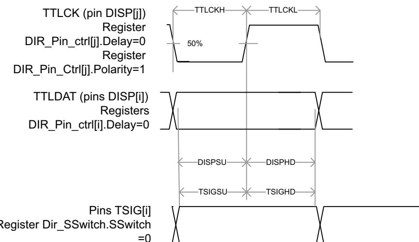
**Figure 2.28. :** TTL operation output timing (2)
