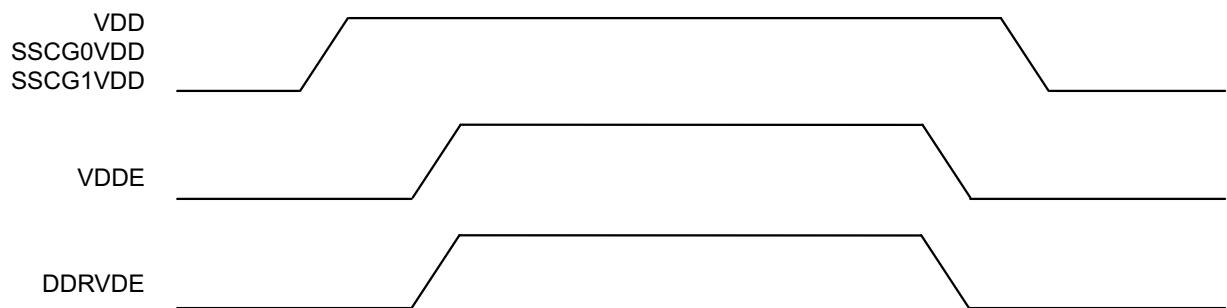
**Figure 2.1. :** The order of recommended power supply
