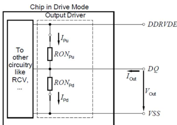
**Figure 2.8.** : Output driver DC characteristics definition
