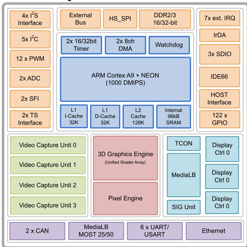
**Figure 1.3. :** MB86R13 block diagram
