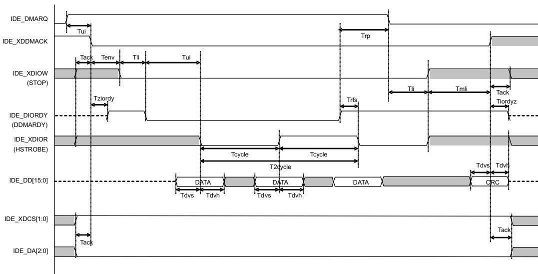
**Figure 2.44. : IDE Write access timing**
