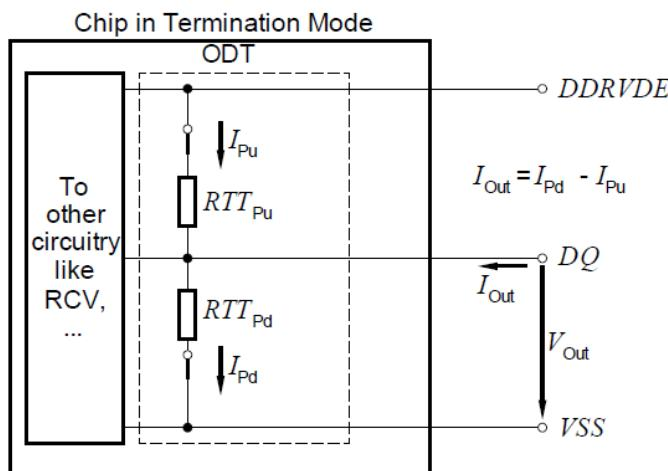
**Figure 2.9. :** ODT DC Characteristics Definition
