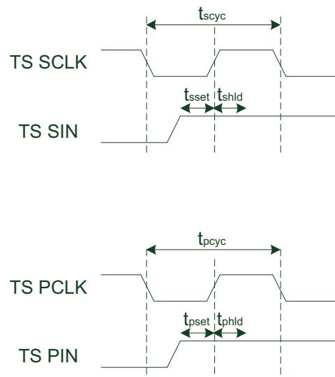
**Figure 2.50.** : TS timing of not inverted mode
