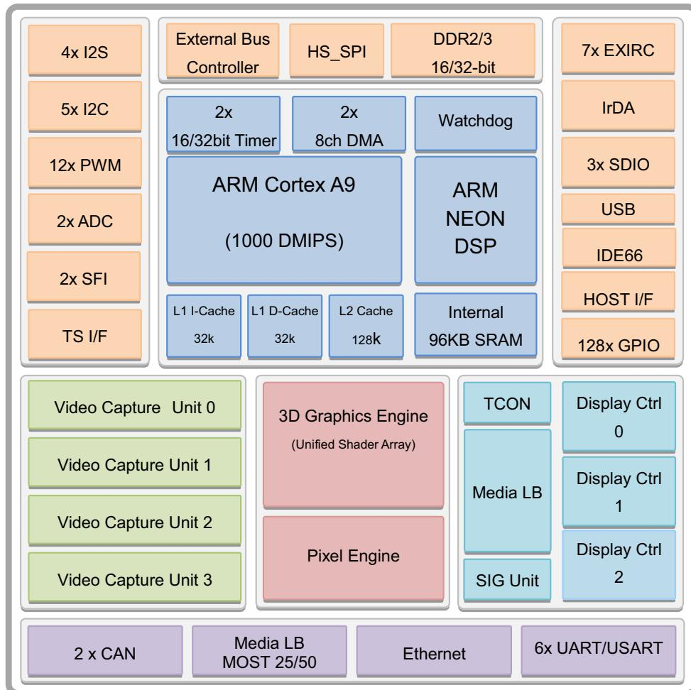
**Figure 1.1. :** MB86R11F block diagram
