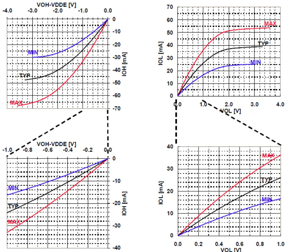
**Figure 2.6. :** 3.3V standard CMOS I/O V-I characteristic (Driving capability 6mA)
