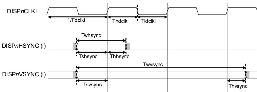
**Figure 2.23.** : Display input signal timing
