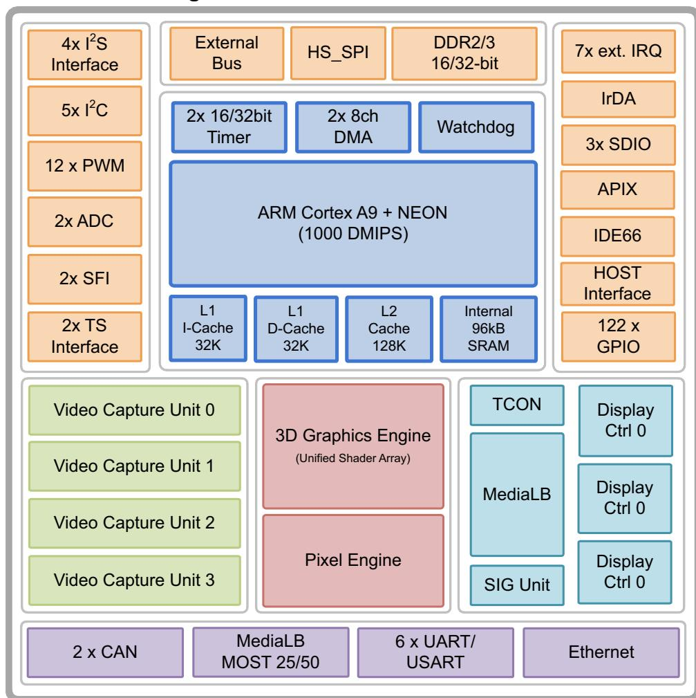
**Figure 1.2. :** MB86R12 block diagram
