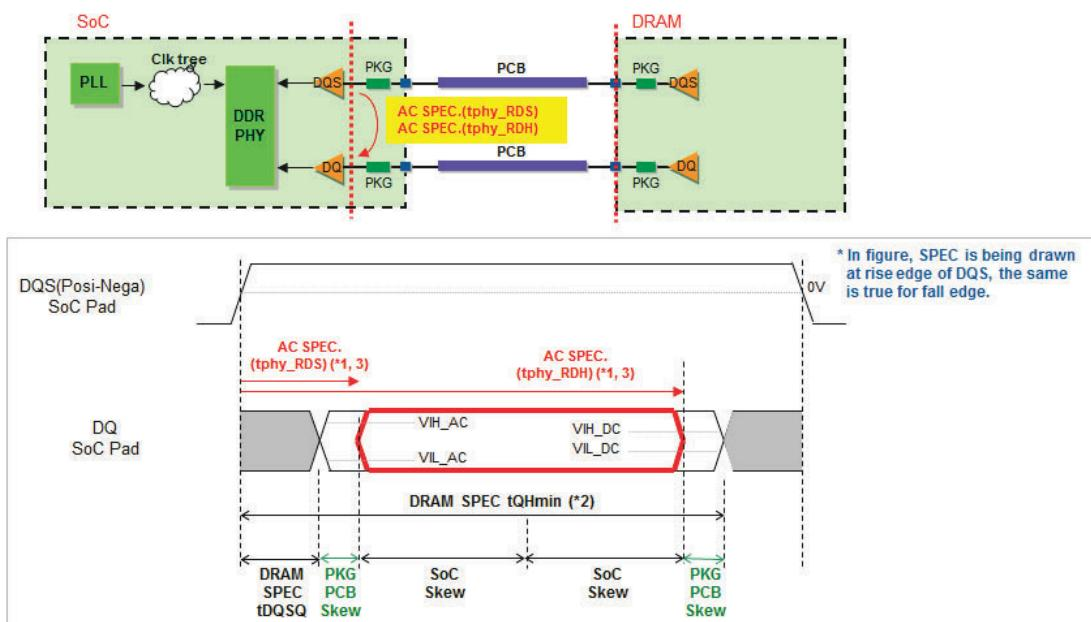
\*1) AC SPEC.(tphy\_RDS/tphy\_RDH) is a constant in spite of input slew. (Derating like DRAM SPEC tDS/tDH is unnecessary.)
