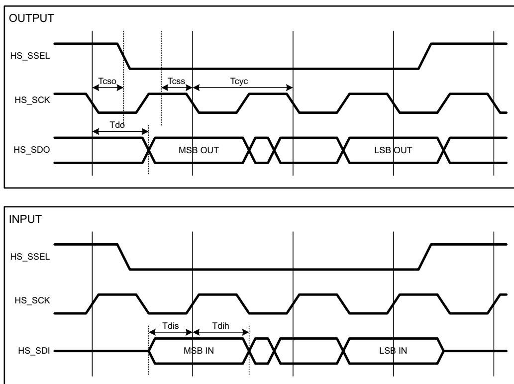
**Figure 2.53.** : HS\_SPI signal timings
