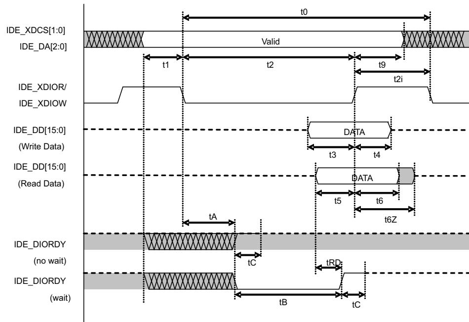
**Figure 2.42. :** PIO access timing
