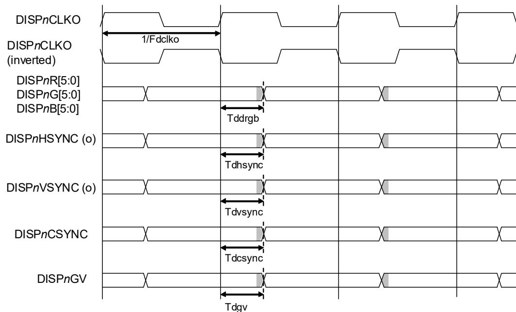
**Figure 2.24. : Display output signal timing**
