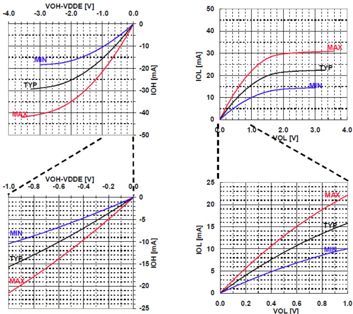
**Figure 2.5. :** 3.3V standard CMOS I/O V-I characteristic (Driving capability 4mA)
