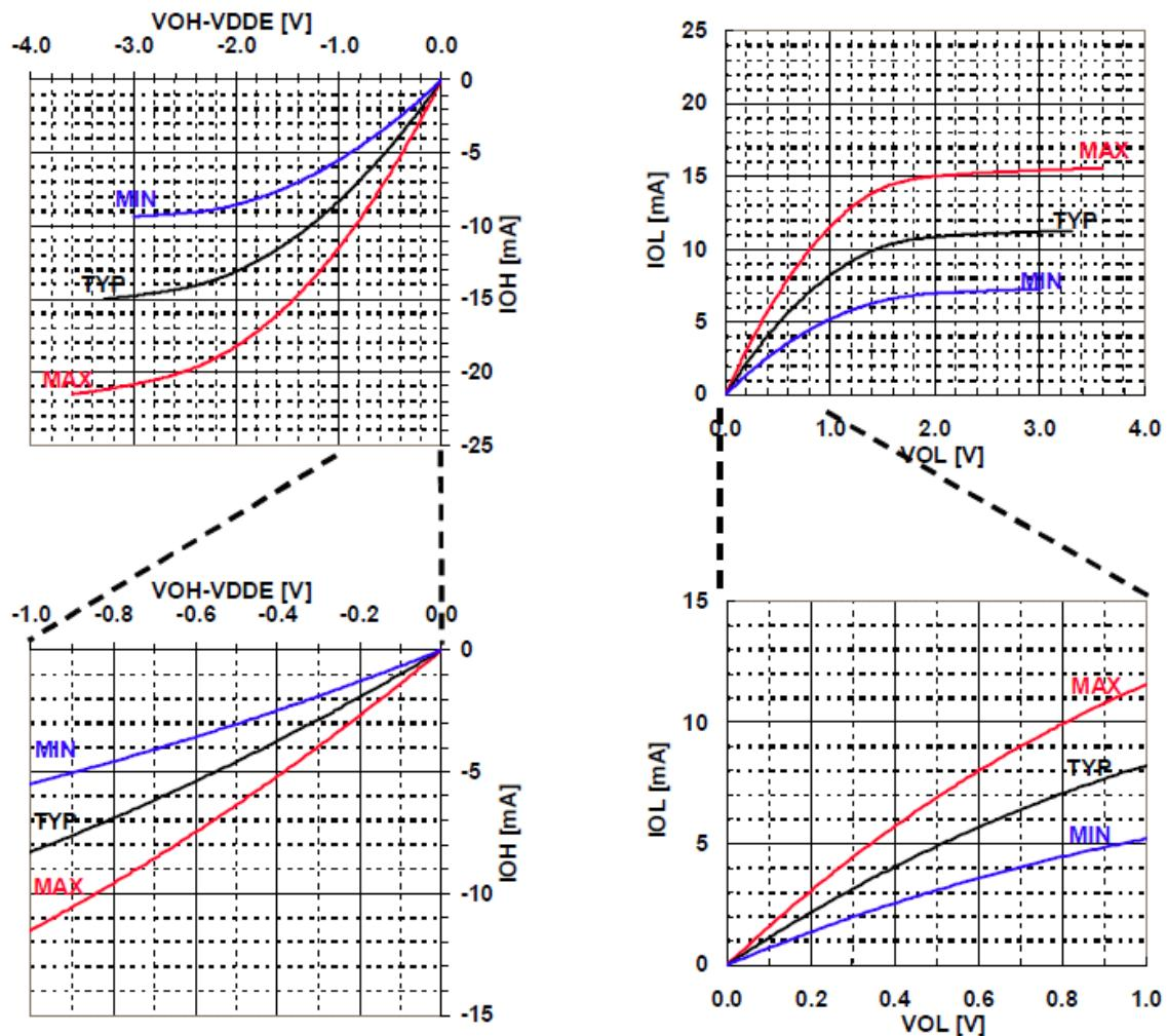
**Figure 2.4. :** 3.3V standard CMOS I/O V-I characteristic (Driving capability 2mA)
