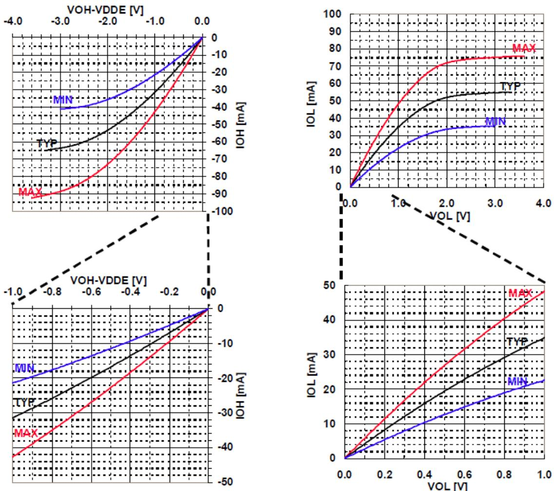
**Figure 2.7. :** 3.3V standard CMOS I/O V-I characteristic (Driving capability 8mA)
