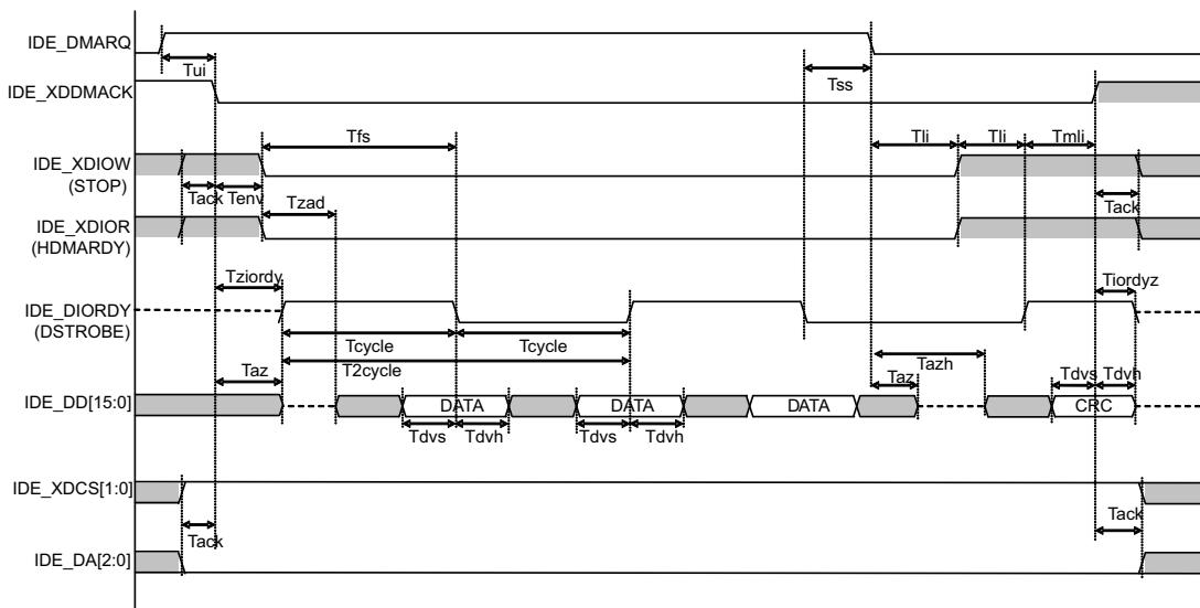
**Figure 2.43. : IDE Read access timing**
