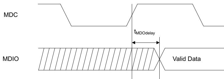
**Figure 2.49.** : MDIO output timing
