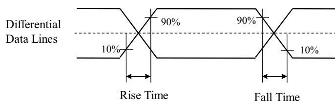
**Figure 2.41. :** Data signal fall and rise time
