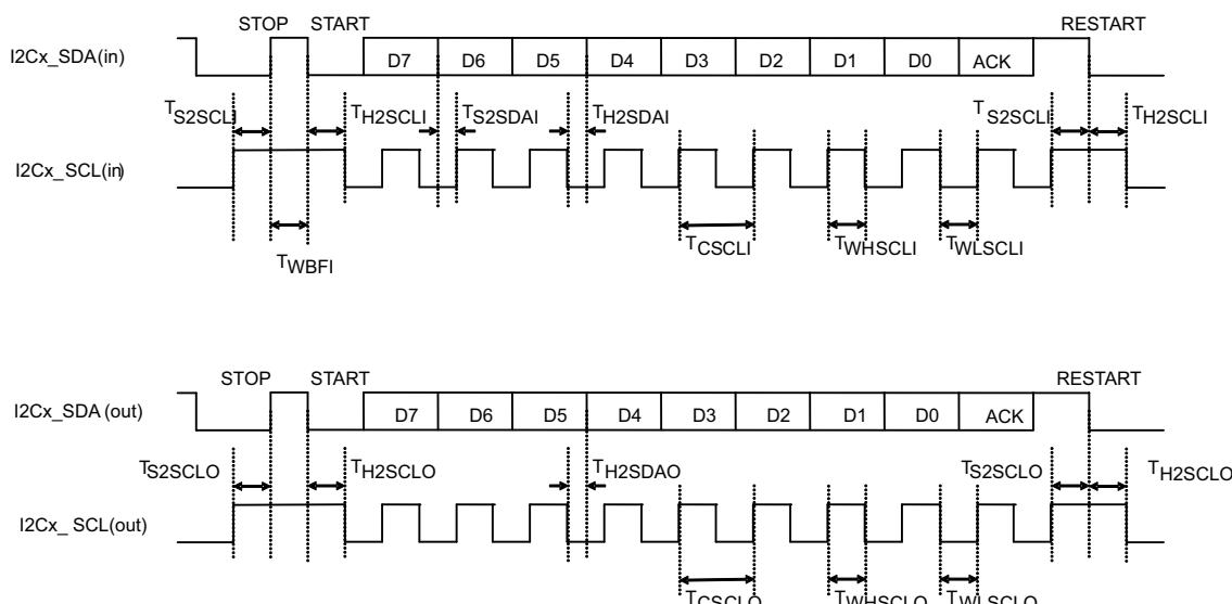
**Figure 2.36.** : I<sup>2</sup>C access timing
