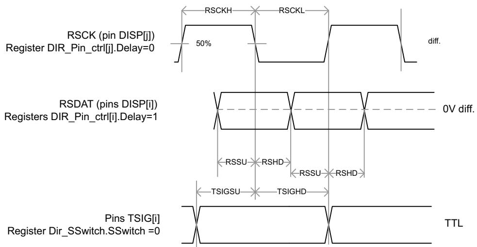
**Figure 2.25.** : RSDS operation output timing
