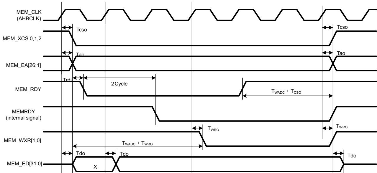
**Figure 2.14. : Low speed device Write**
