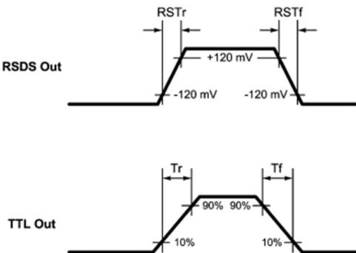
**Figure 2.26.** : RSDS/TTL operation output timing
