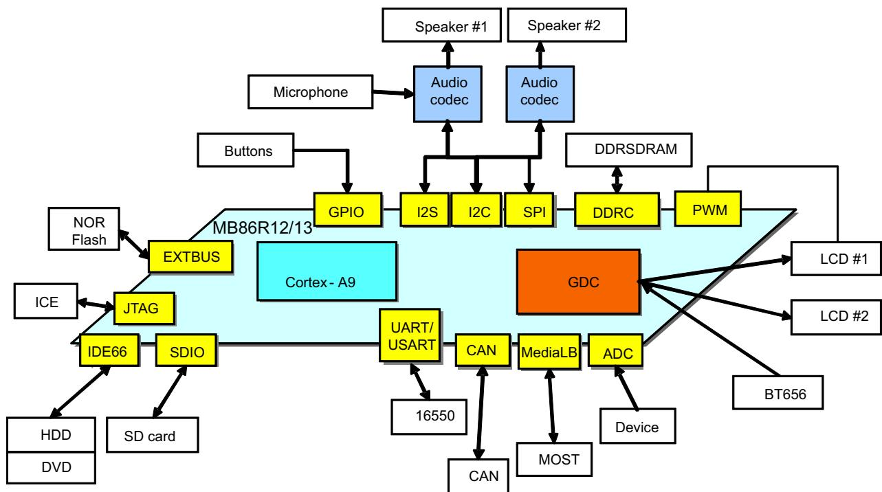
**Figure 1.5. :** MB86R12/13 system configuration
