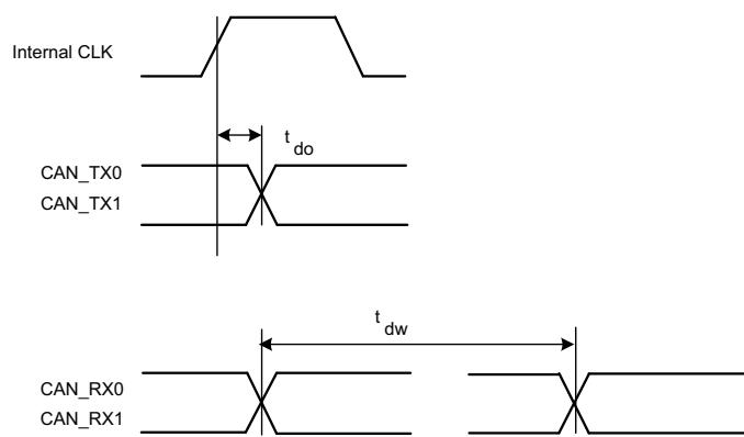
**Figure 2.38.** : CAN timing
