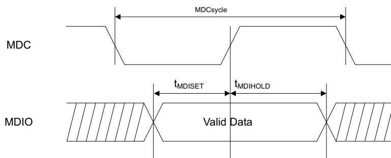
**Figure 2.48.** : MDIO input timing
