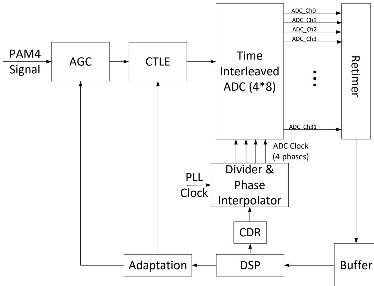
**Figure 2. ADC-DSP Receiver Block Diagram.** The specific receiver shown here is implemented with a 4\*8 ADC configuration, i.e., 4 parallel and interleaved ADC blocks, with 8 sub-ADC blocks in each ADC. The ADC is driven by a 4-phase clock that is generated from the PLL clock. The ADC configuration can be adjusted based on the desired ADC clock speed.
