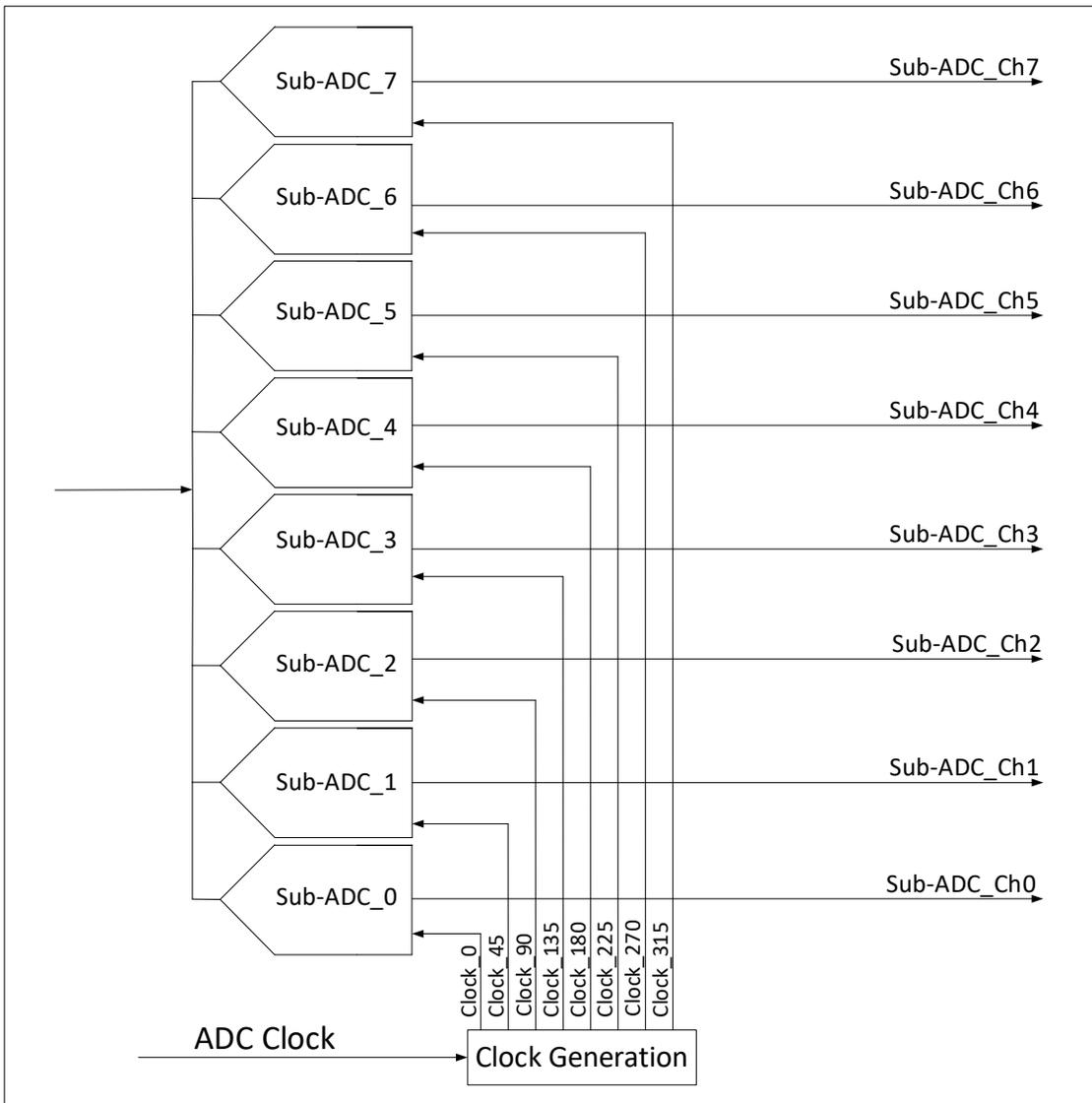
**Figure 4. Sub-ADC Implementation within each ADC unit. In this case, 8 sub-ADC units are implemented and clocked with 8 equally spaced (45 degree) phases of the ADC clock.**
