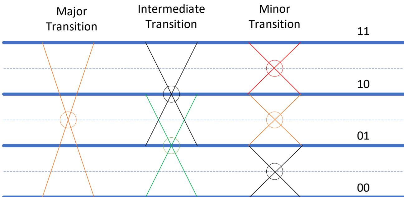
**Figure 1. Transitions for PAM4 signaling. The major transition is the change between 00 <-> 11. The intermediate transitions are the changes between 00 <-> 10, and 01 <-> 11. The minor transitions are the changes between 00 <-> 01, 01 <-> 10, and 10 <-> 11.**
