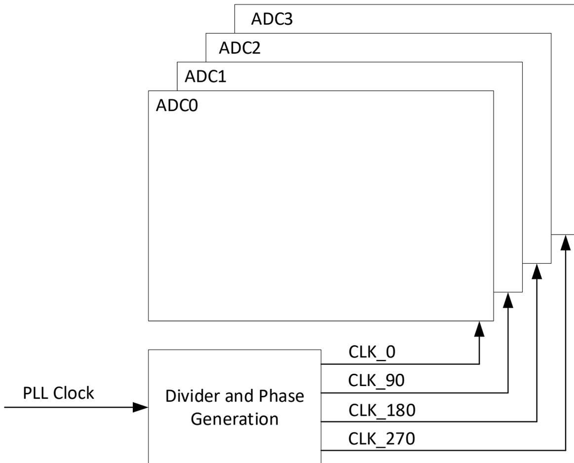
**Figure 3. Parallel ADC Implementation. In this case, four parallel ADC blocks are implemented, and clocked with four equally spaced (90 degree) phases of the PLL clock.**
