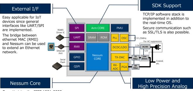
By optimizing the IEEE 1901-2020 conforming Nessum core for IoT devices, design area and BOM can be reduced.
